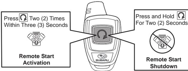
**NOTE: All vehicle doors, hood, trunk or rear gate must be closed prior to activating the remote engine start system. Any open entry point will prevent starting or cause the system to shut down.**
